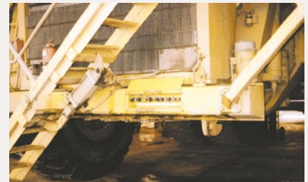
Service Box Fitted to Heavy Haul Mine Vehicle
